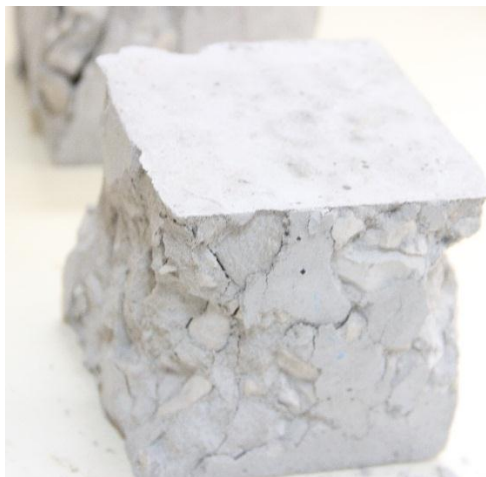
Figure (3.6): crushed compressive testing cube after failure.
