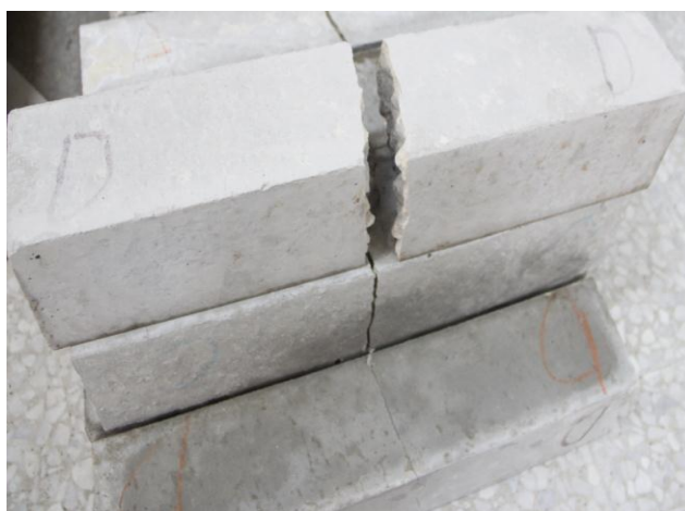
Figure (3.7): Crushed concrete cubes and prisms.
