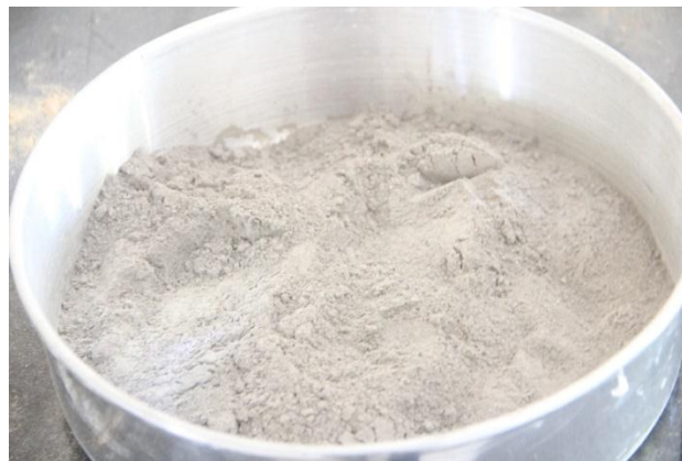
Figure (3.4): Glass powder particles (less than 75 \mu\text{m} ).
